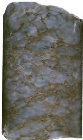
Borehole core of HARTLEPOOL ANHYDRITE made by the drilling rig
