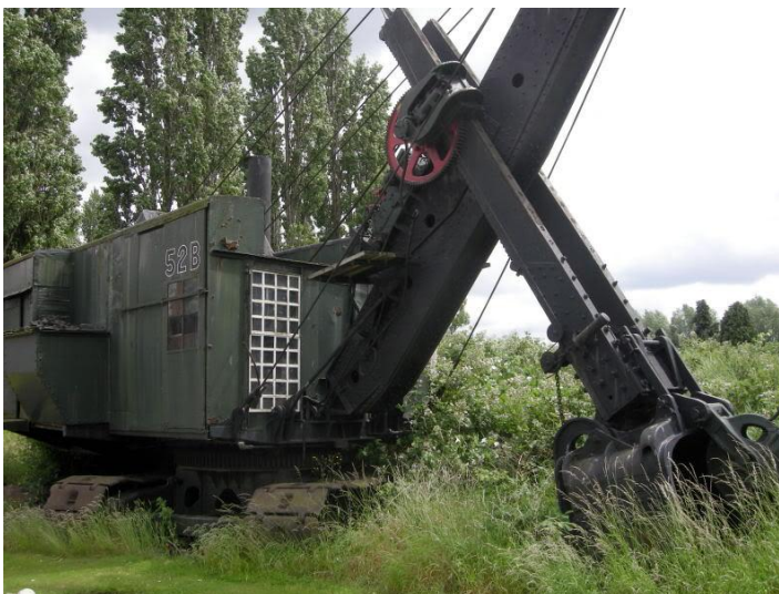
Fig 5: Ruston Bucyrus Excavator of the type used in World War II
