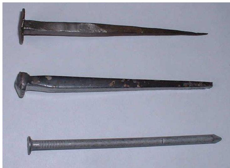
Fig 10 Nail Types: From top to bottom, Handmade, Cut and Wire or French Nail.
