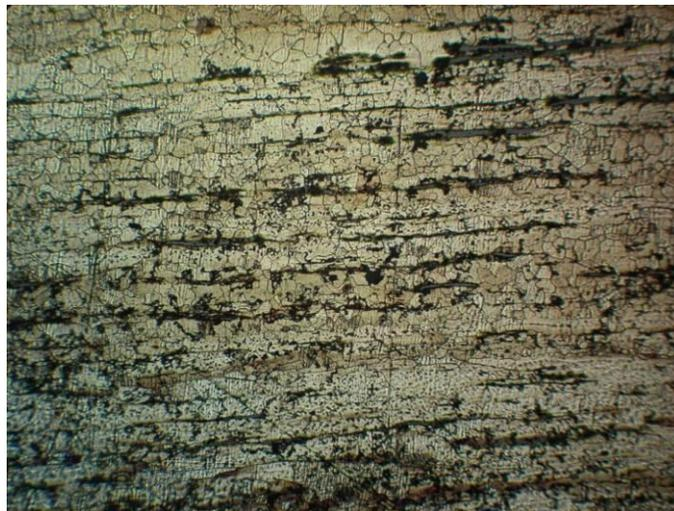
Fig 7 SEM image Wrought Iron etched in 2% Nital
