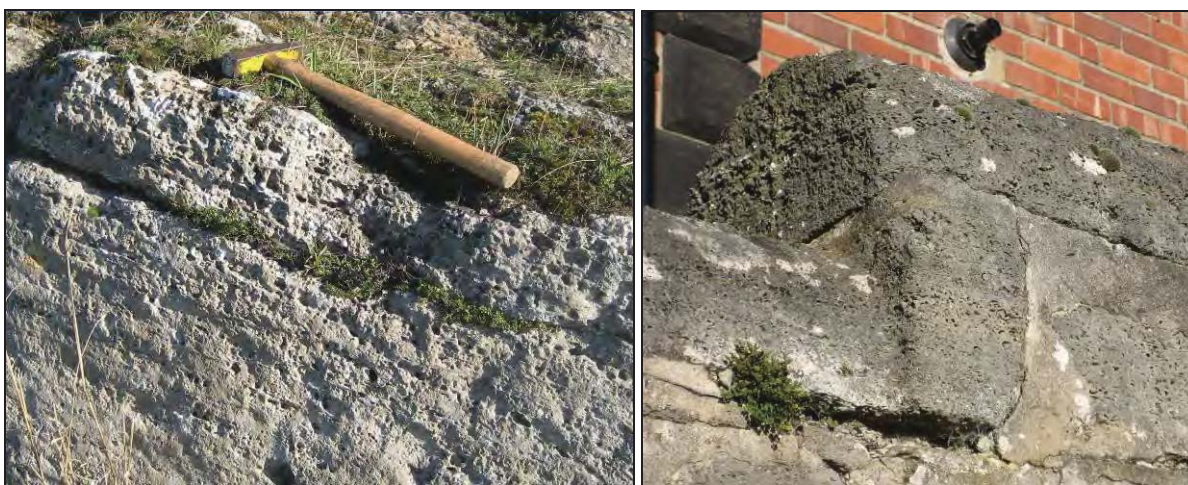
Plates 12 and 13: Sponge-like Concretionary Limestone exposure in old quarry on Cleadon Hills, and utilised in the boundary wall of Cleadon Waterworks.
